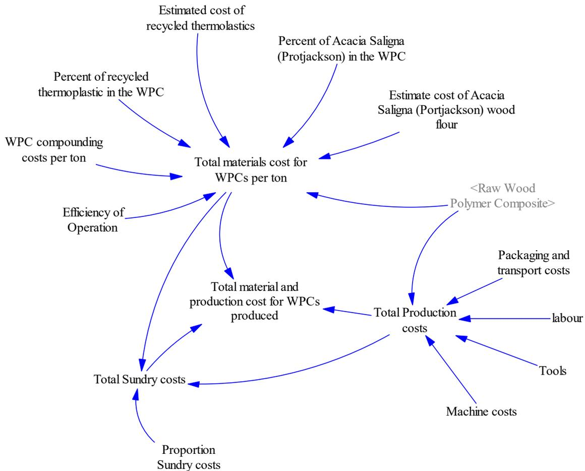
**Figure A4: The cost sub-model of the establishment of the WPC production plant**
